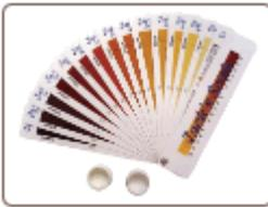
The Honey Color Grader has a chart with Pfund (0-140mm). It's easy to use, all you do is fill the provided cup and use the chart to compare. There is no electricity needed. Pocket size, 2" x 8.5".
