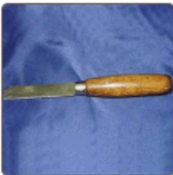
This Section Scrapping Knife is specially designed and constructed for cleaning wax and propolis from finished sections.
