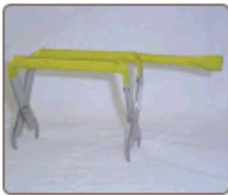
This handy tool, imported from Portugal, features a combination frame manipulation tool and frame grip all in one. Loosen the frame with the tool end then grip.
